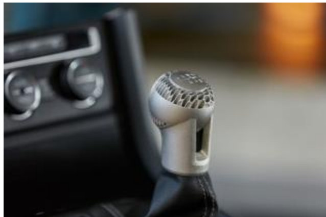
Figure 6: An example of an automotive component produced by MBJ (Image source: HP [34]).
